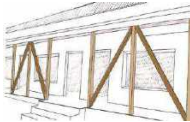
12. Timber diagonal braces between timber posts in "K" configuration. They are placed where they don't obstruct movement.
