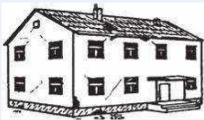
Grade 2: Moderate damage
