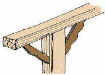
14. Timber Knee braces. They are not as effective as diagonal braces. But they permit unhindered movement of people.
