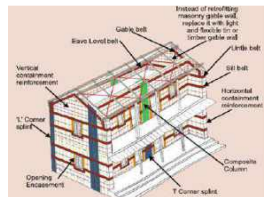
Figure 9: Key elements in splint and bandage approach (Source: UNDP)
