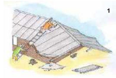
Damaged roof because of severe damage to the support walls and other support systems.
