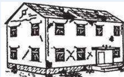
Grade 3: Substantial to heavy damage
